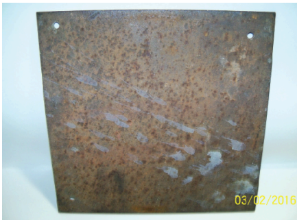
This untreated steel panel shows excessive rust after 10 years of outdoor exposure.
