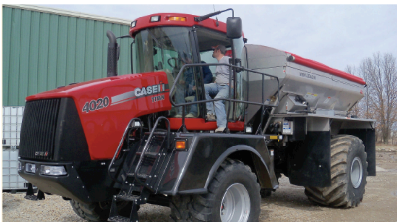
This CASE dry fertilizer applicator sells for approximately $300,000. According to Deardorff, it will have a trade-in value of less than $10,000 and a service life of less 10 years due, in large part, to corrosion and wear.
