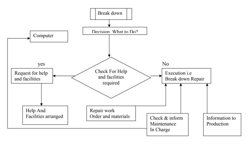
**Corrective Maintenance**: his Maintenance is carried out for restoring a failed unit. May be little repair to re-design of equipment. It is very fast process. Thus it included in both planned and unplanned **Maintenance**. Work out to eliminate the offline jobs of lower order priority and to eliminate /reduce repetitive breakdown.
