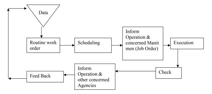
**Preventive Maintenance**: This is one of the oldest method maintenace. Today also it is used mostly along with corrective main Maintenance and Condition Based Maintenance
