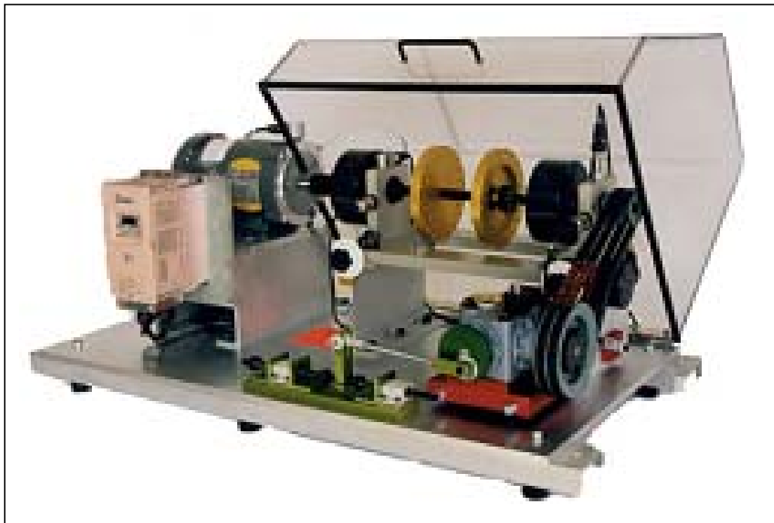
Figure 1. A snap shot of Spectra Quest's Machinery Fault Simulator used in the study.
