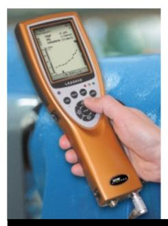
Many ways to get relevant data: broadband vibration, shock pulses, spectrum analysis, speed, temperature, other signals in voltage or current, all from one instrument weighing only 600 grams. A 206 MHz Intel® StrongARM\* processor crunches numbers to work out the easy answer: green for good, yellow for caution, red for bad.
