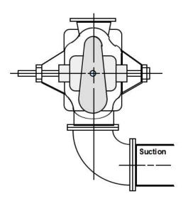
Under these conditions, the overloaded bearing will fail prematurely and regularly if the pump is packed. If the pump is fitted with mechanical seals, the seal will usually fail instead of the bearing--but just as regularly and often more frequently. When it is absolutely essential to position an elbow on the inlet of a double suction pump, it must be located at right angles to the shaft.
