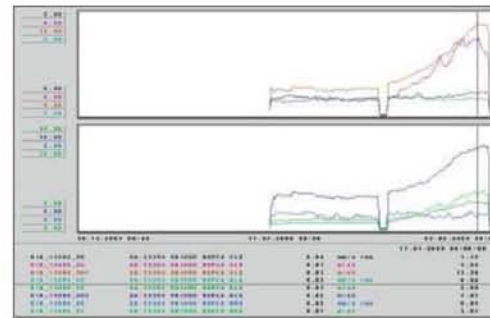
Figure 5 - PMS screen showing trends of gearbox high-speed shaft upper and lower bearing vibration, filtered to various frequencies and with various signal conditioning applied.
