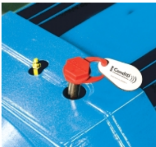
Fig 3: Adapter for shock pulse measurement with electronic ID tag
