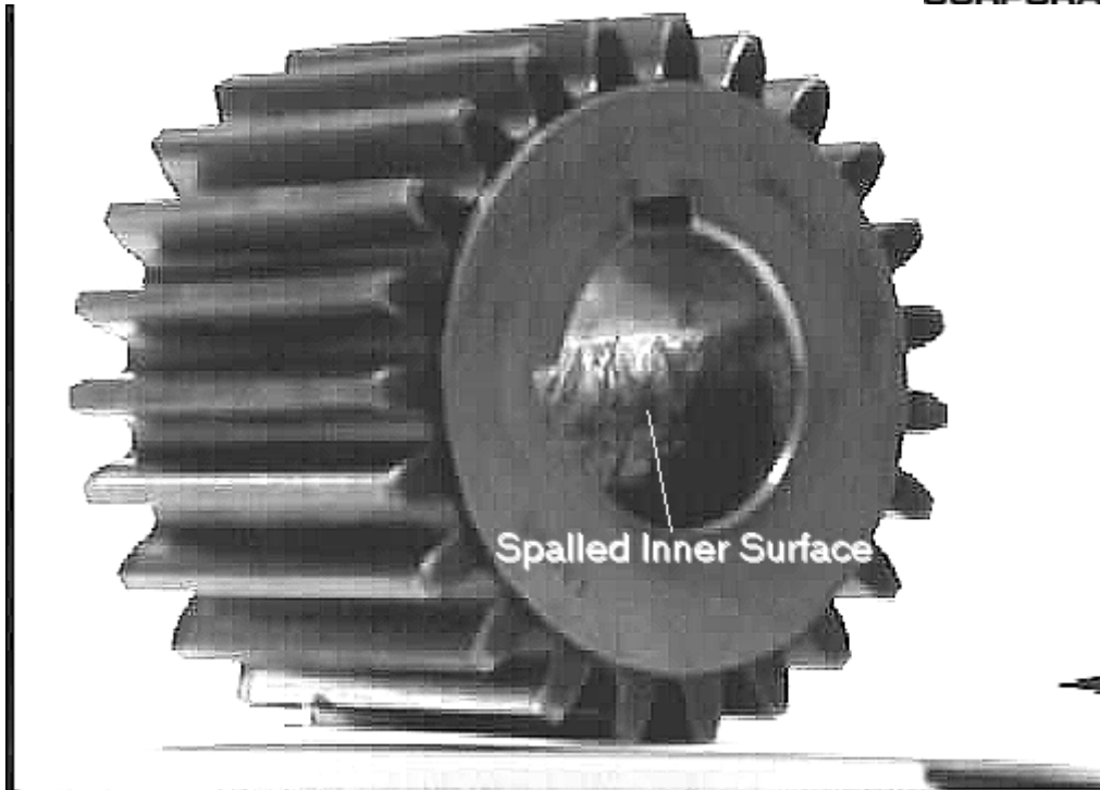
The figure above shows the spalling in the pinion bore caused by the gear turning back and forth on the shaft.
