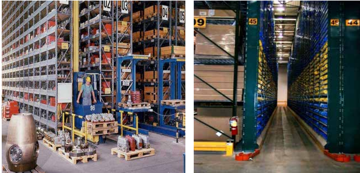
Figure 4 – Parts Storage in Narrow Aisle Shelving
