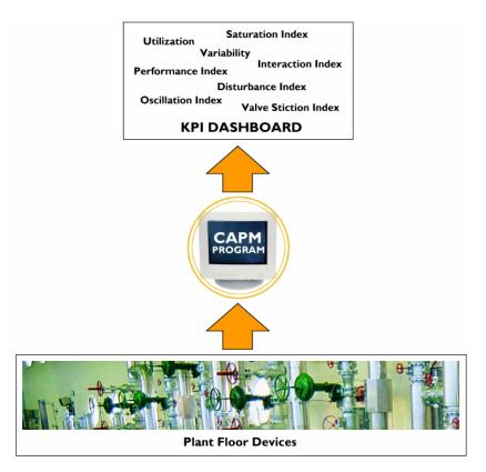
Figure 2: CAPM applications capture plant floor data to create KPIs
